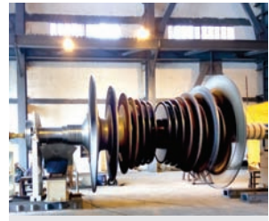
On Site field Balancing of 600 MW LP Rotor
