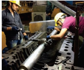
In-situ machining of sealing fins on inner casing and on HP rotor of 200 MW
