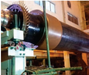
On site field Machining 1060 MW Generator rotor
