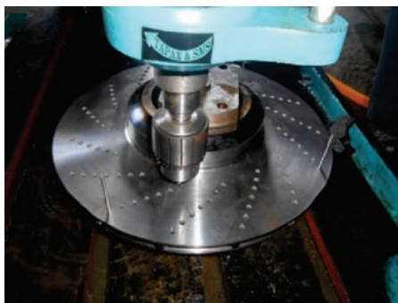
Drilling & Reaming of impeller disc lock pin holes
